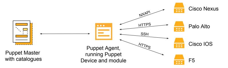
Modules from: Cisco Nexus, Palo Alto, Cisco IOS, F5 Big-IP, Cisco ACI, Cisco Meraki, Netscaler, NetApp, Huawei, Arista, Cumulus, Lenovo CNOS
