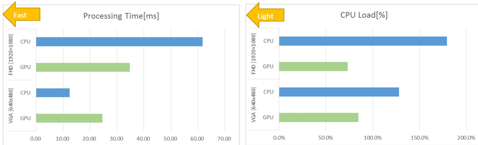
**Longer processing time but lower CPU load by "128% -> 85%" in VGA.
