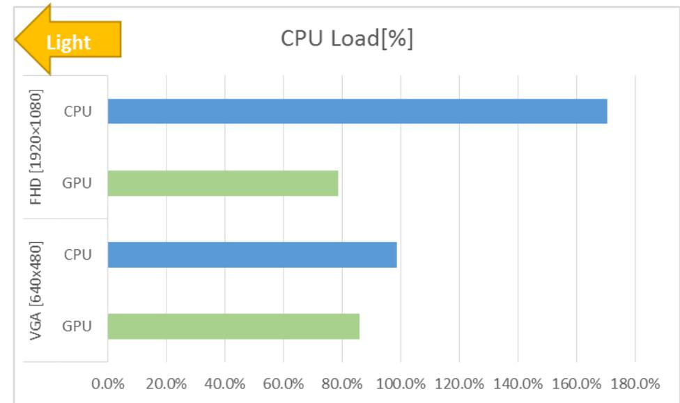
**Longer processing time but lower CPU load by "99% -> 86%" in VGA. Shorter processing time by "74ms -> 35ms" and lower CPU load by "170% -> 78%" in Full-HD and GPU effects work for both!**
